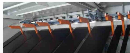
Lever type pneumatic sheet support system (optional) Avoids hanging down the wide and thin sheets via pneumatic arms support and provides more precise cuts.
